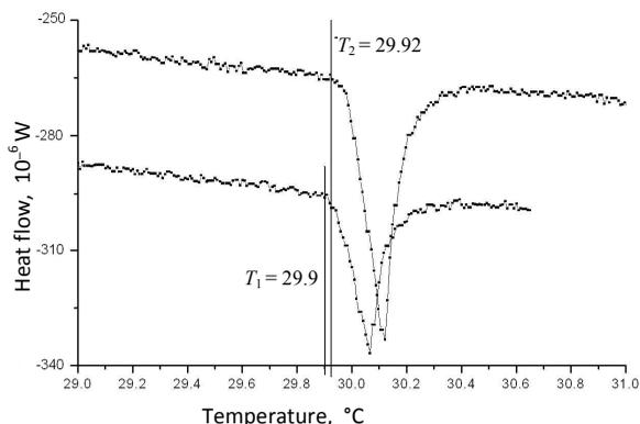
**Fig. 2.** A thermogram of heating a temperature reference sample (1 mg Gallium, 29.9 °C) in the calorimetric chambers at a rate 0.2 K/min
