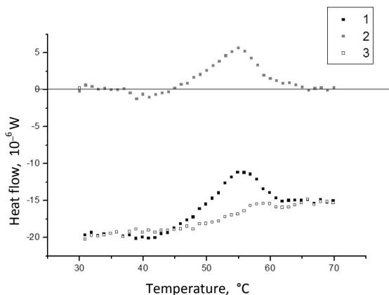
**Fig. 3.** Heat denaturation of ovalbumin in the temperature-modulation mode StepScan. 1 —  $P$ , 2 —  $f(T,t)$ , 3 —  $C_p(dT/dt)$  for the process under study
