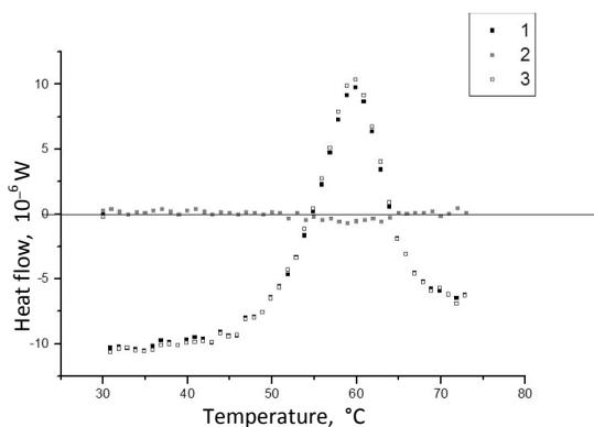
**Fig. 4.** Heat denaturation of lysozyme in the temperature-modulation mode StepScan. 1 —  $P$ , 2 —  $f(T,t)$ , 3 —  $C_p(dT/dt)$  for the process under study.
