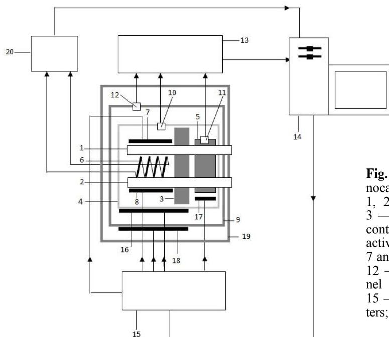
**Fig. 1.** Functional diagram of a modulation nanocalorimeter.
